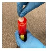
At the end of sample collection in BR, disconnect the dust collector from the vacuum cleaner hose by twisting or pulling. Place the small top cap on first and place the
